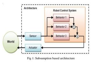
The behavior based robots need information about the world so they can relate themselves to the environment, just like animals. For this purpose, they rely on sensor devices which transform the world stimuli into electrical signal. These signals are electrical data which represents state of about the world and must be interpreted by the robot to achieve its goals.
